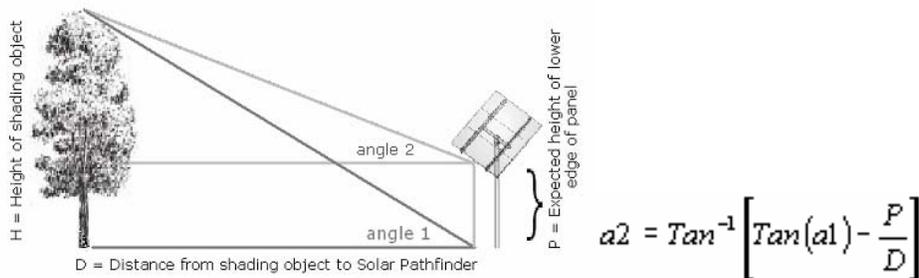
**To estimate needed height (pole mount) to overcome shading:**
